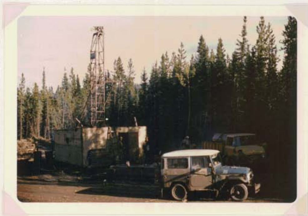
Photo 10. Canadian Lonyear's skid-mounted "44" diamond drill on drillsite #9. Unimog water truck in background.
