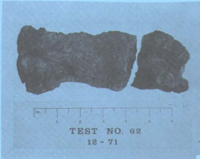
Figure 7 - 30% Saxon No. 3 +70% Reference H.V. Coal
