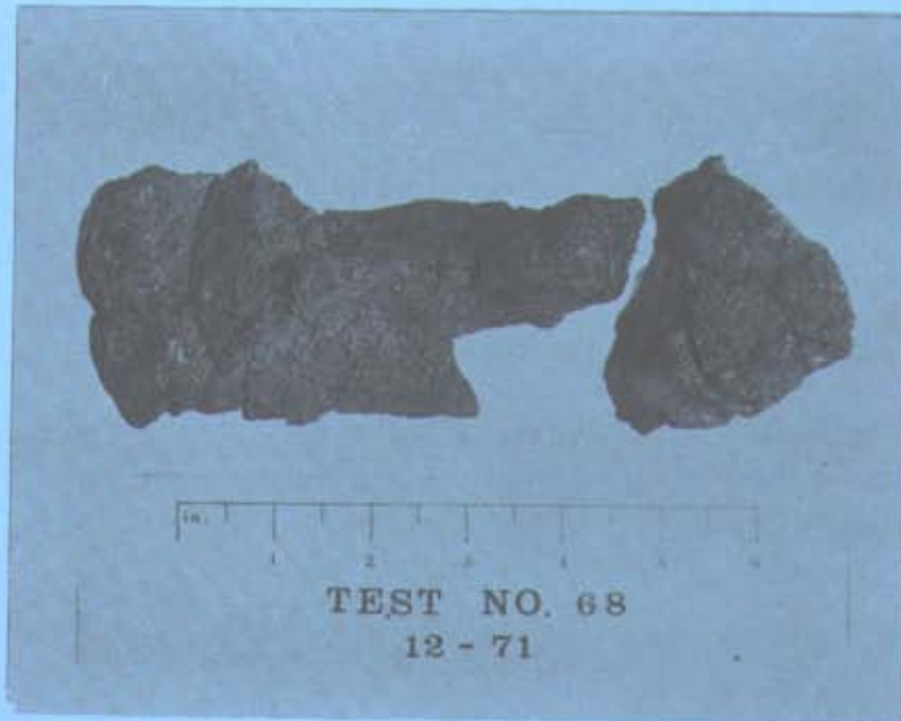
Figure 5 - 30% Saxon No. 1 +70% Reference H.V. Coal
