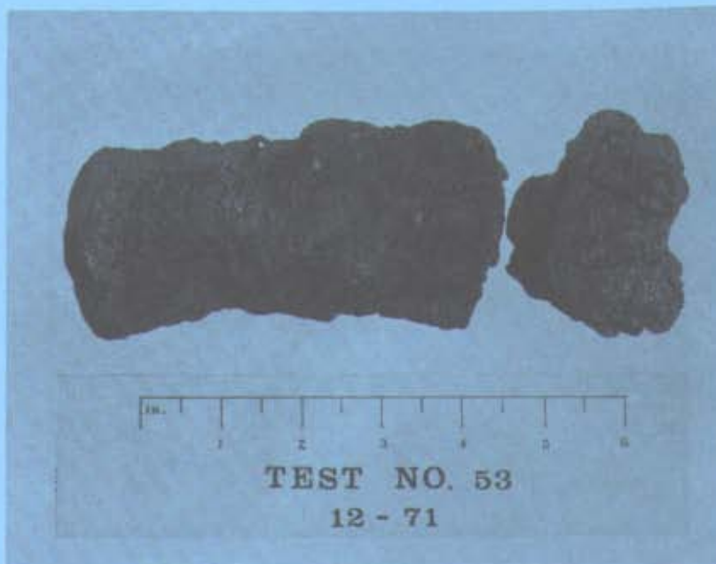
Figure 6 - 30% Saxon No. 2 +70% Reference H.V. Coal
