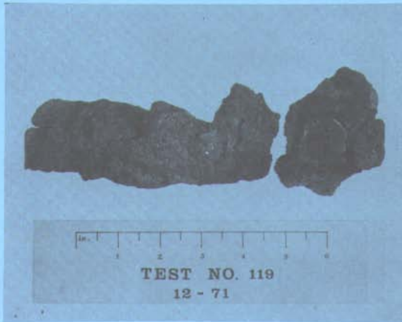
Figure 8 - 30% Saxon No. 4 +70% Reference H.V. Coal
