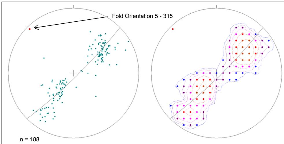
*Figure 7.6: Stereonet plots of all South Ridge structural mapping data*
