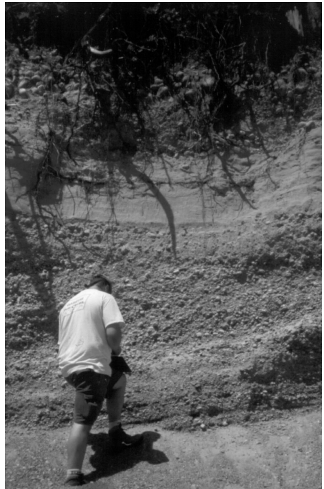
Photo 4. Typical sediments found along the Sunshine Coast in aggregate pits. They consist of interbedded sand, sandy gravel and gravel associated with a relict delta.
